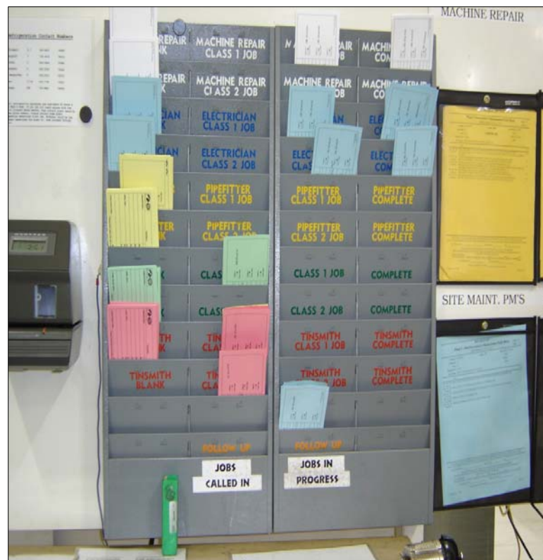
Cell leaders punch in machine problems as part of the andon response system. The colored cards correspond to different trades.
